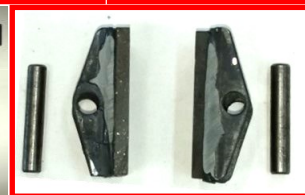
High Temperature Brake Pads Heat Bonded to Shoes & Pins
